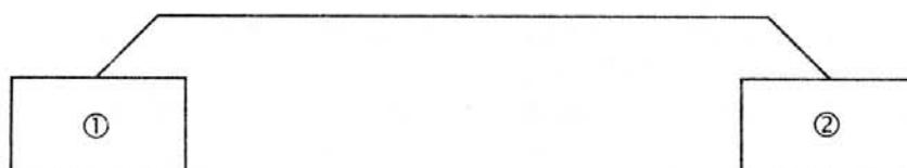
1) FX<sub>2N</sub>, FX<sub>2NC</sub> (可屏蔽双绞线)
