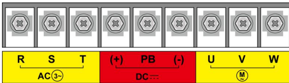
图 4-4 EC160+电梯智能整体机主回路端子排的布局(18.5kW~30kW)
