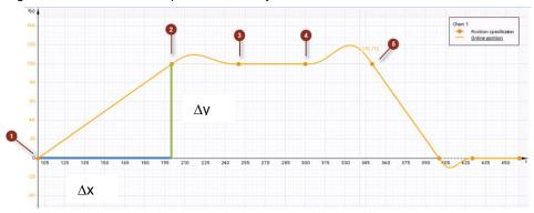
Figure 4-2: Configuration of cam with 8 points created by LCamHdl\_CreateCamBasic
