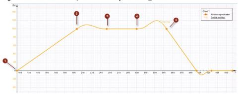
Figure 1-4: Configuration of cam with 8 points created by LCamHdl\_CreateCamBasic
