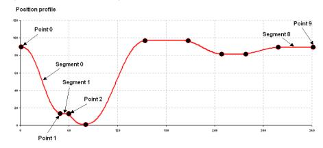
To define the cam segments all points and their dynamics (1st and 2nd geometric derivation) have to be specified.
