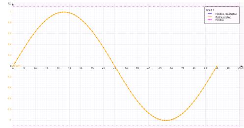
Figure 1-6: Cam disk example (interpolation mode C splines) created by LCamHdl\_CreateCamBasedOnXYPoints
