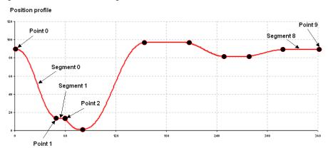
Figure 1-1: Cam disk consisting of several elements
