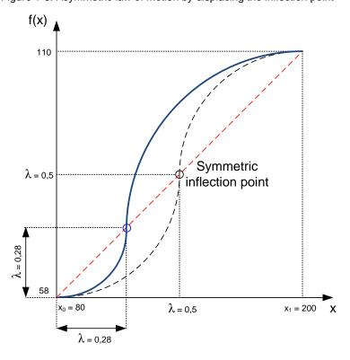
Figure 1-8: Asymmetric law of motion by displacing the inflection point
