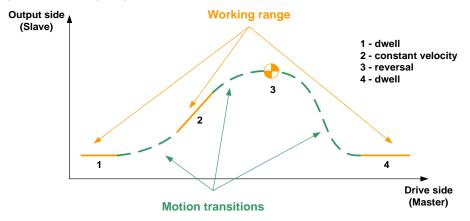
A motion transition between two consecutive working ranges has to fulfill boundary conditions (Figure 4-7), e.g. velocity and acceleration has to be continuous. This guarantees that the drive runs smoothly, e.g. without jerks. The elements are described by mathematic functions between start and end point, e.g. polynomials.
