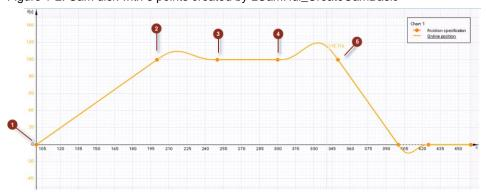
Figure 1-3: Configuration of cam with 8 points created by LCamHdl\_CreateCamBasic
