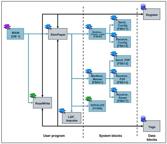
The core functionality includes the function block "EbmPapst". This block is called in the cyclic organization block "Main". The interfaces of FB "EbmPapst" are fed from the data blocks
