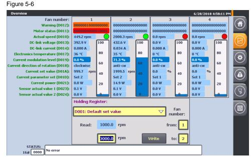
Depending on which operating mode is set (holding register D106/D107), the current set value (D01A) is displayed in the unit "rpm" for speed control and in "%" for control.
