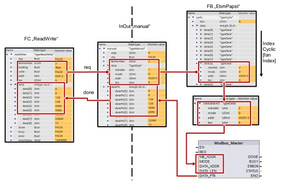
The task is transmitted to the FC "ReadWrite" via the following input parameters:
