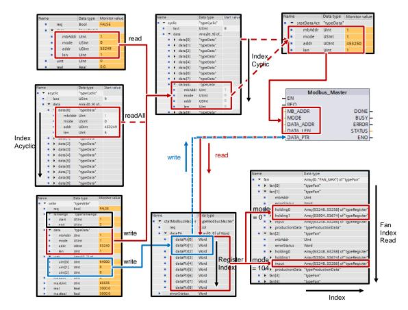
The sequence for reading the input registers of each fan is processed cyclically as a function of the running index "IndexCyclic". The information (access mode "mode", register address "addr" and register length "len") are provided as start values in the interface parameter "cyclic" in the field 0 to 7.
