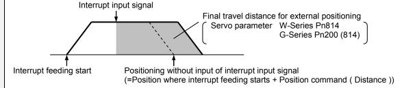
The Positioning completed (Done) is turned ON when the positioning operation for the FB has been completed. This Flag is also turned ON when the positioning operation is completed without the interrupt feeding signal input. This flag will not be turned ON if the positioning operation is canceled because another operation has been started from a different instance, for a deceleration stop, or because an error has occurred.
