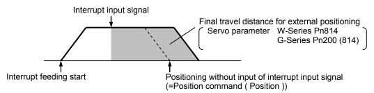
The Positioning completed (Done) is turned ON when the positioning operation for the FB has been completed. This Flag is also turned ON when the positioning operation is completed without the interrupt feeding signal input. This flag will not be turned ON if the positioning operation is canceled because another operation has been started from a different instance, for a deceleration stop, or because an error has occurred.
