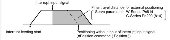
The Positioning completed (Done) is turned ON when the positioning operation for the FB has been completed. This Flag is also turned ON when the positioning operation is completed without the interrupt feeding signal input. This flag will not be turned ON if the positioning operation is canceled because another operation has been started from a different instance, for a deceleration stop, or because an error has occurred.
