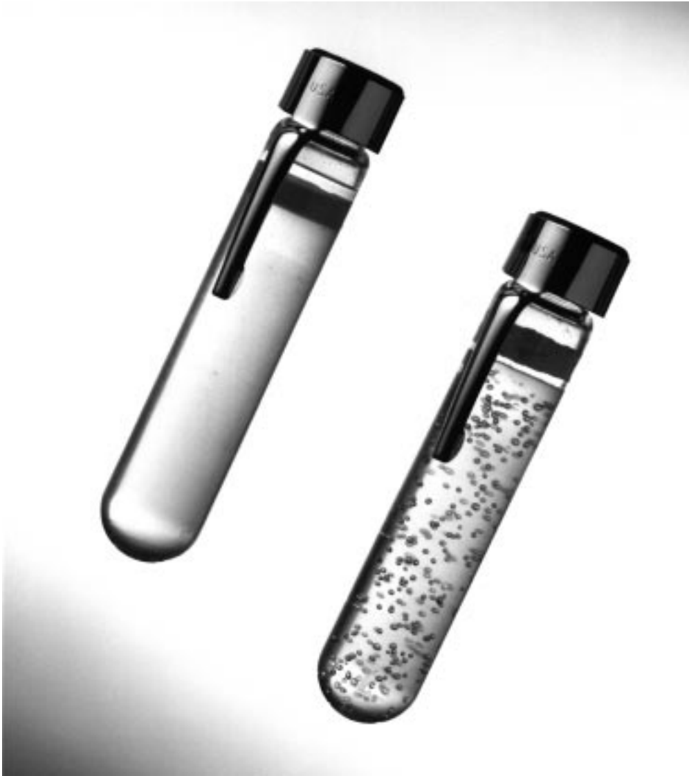
FIGURE 69.5 Bubble dosimeters for personal dosimetry of fast neutrons. The dosimeter on the left is shown before exposure to fast neutrons. For comparison, a dosimeter exposed to fast neutrons is shown on the right. Bubbles are clearly evident throughout the volume of the dosimeter. (Courtesy of Siemens Medical Systems, Inc.)
