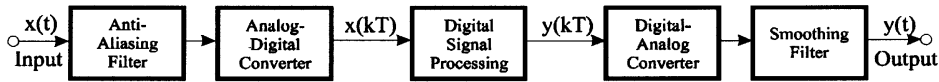
FIGURE 82.16 A data acquisition system with continuous time inputs and outputs uses antialias prefiltering, an A/D converter, digital signal processing, a D/A converter, and an output smoothing filter.
