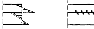
FIGURE 32.2 Bending of bimetallic strip uniformly heated with \alpha_2 \geq \alpha_1 . (a) Bimetallic strip. A_1B_1-A_2B_2 is an element cut out from the strip. (b) Bending of the element A_1B_1-A_2B_2 when uniformly heated. Assuming \alpha_2 > \alpha_1 , the deflection is convex up. The total force acting over the section of (1) is an axial tensile force P_1 and bending moment M_1 , whereas over the section of (2) it is an axial compressive force P_2 and bending moment M_2 . (c) Sketch of the internal resulting stress distribution. (Left): normal stresses over the cross section of the strip. The maximum stress during heating is produced at the interface between the two components of the strip. This stress is due to both axial force and bending. (Right): shearing stresses at the ends of the strip.
