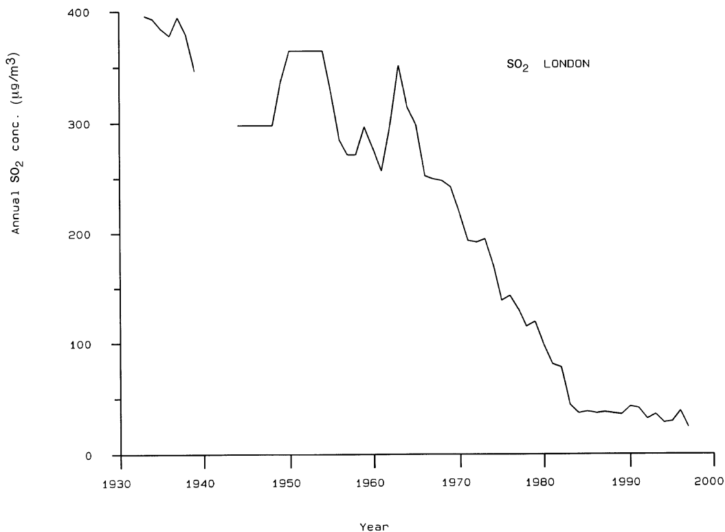
FIGURE 73.7 Annual average SO 2 concentrations in Central London, 1933–1997. The curve shows the average from two sites.
