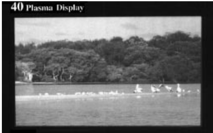
FIGURE 93.3 The 40-in. diagonal dc driven plasma display from NHK. (From Mikoshiba, S., Inf. Display , 10(10), 21, 1994. With permission.)
