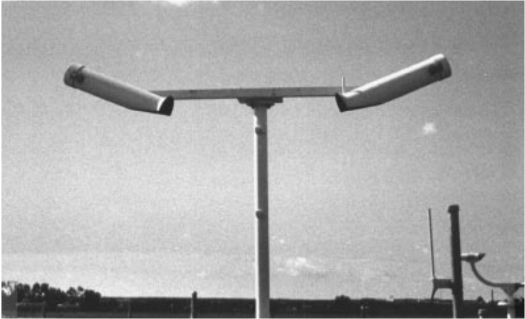
FIGURE 73.5 The xenon flash instrument that determines atmospheric visibility at an ASOS system station. This system is produced by AAI Systems Management Incorp.
