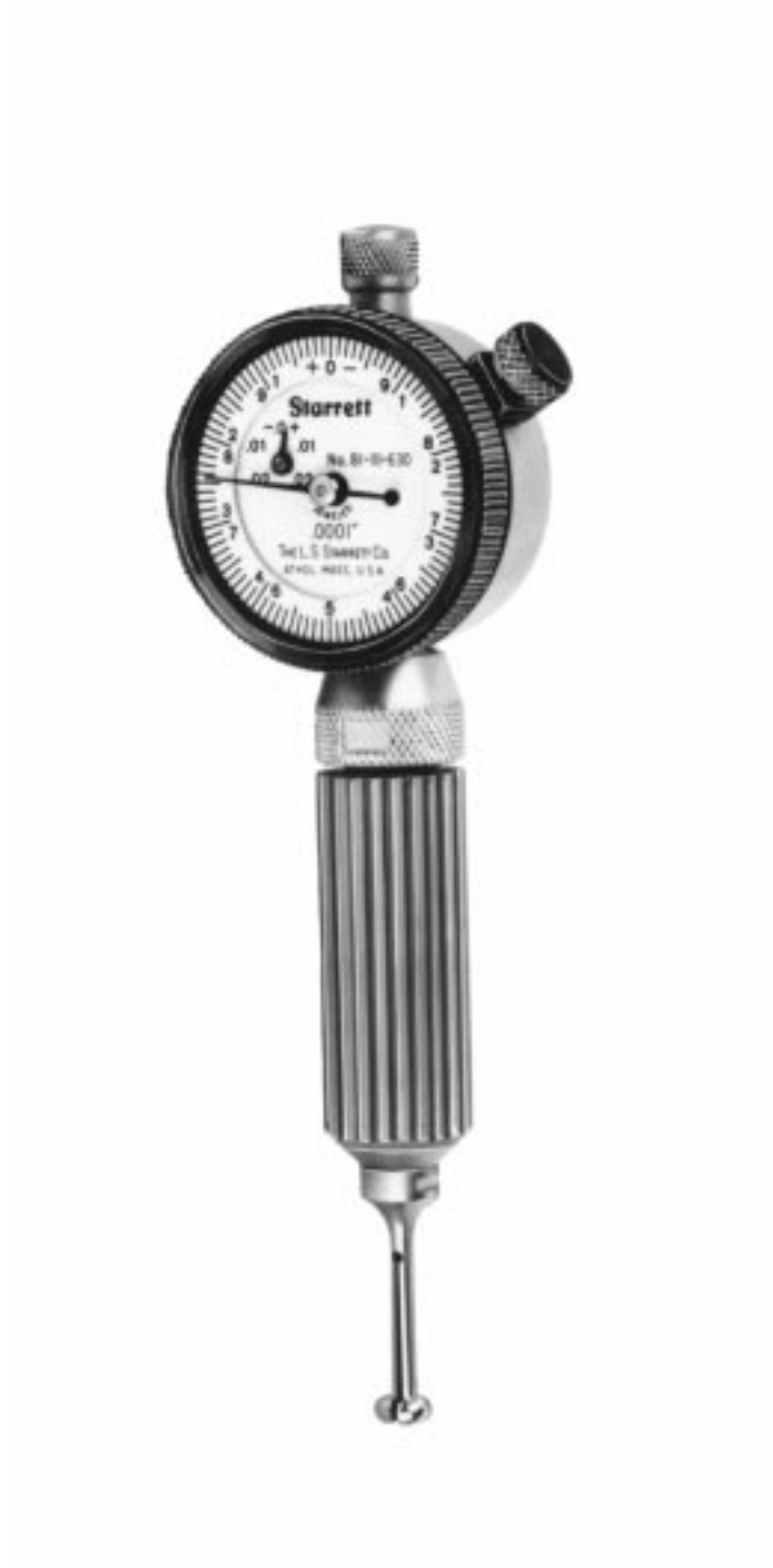
FIGURE 6.54 Industry's most popular dial and electronic bore gages (Courtesy of The L.S. Starrett Co.).
