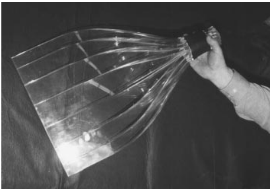
FIGURE 67.6 Photograph of adiabatic Plexiglas light guide. (Courtesy of Science and Technology Centre, Carleton University, Ottawa.)
