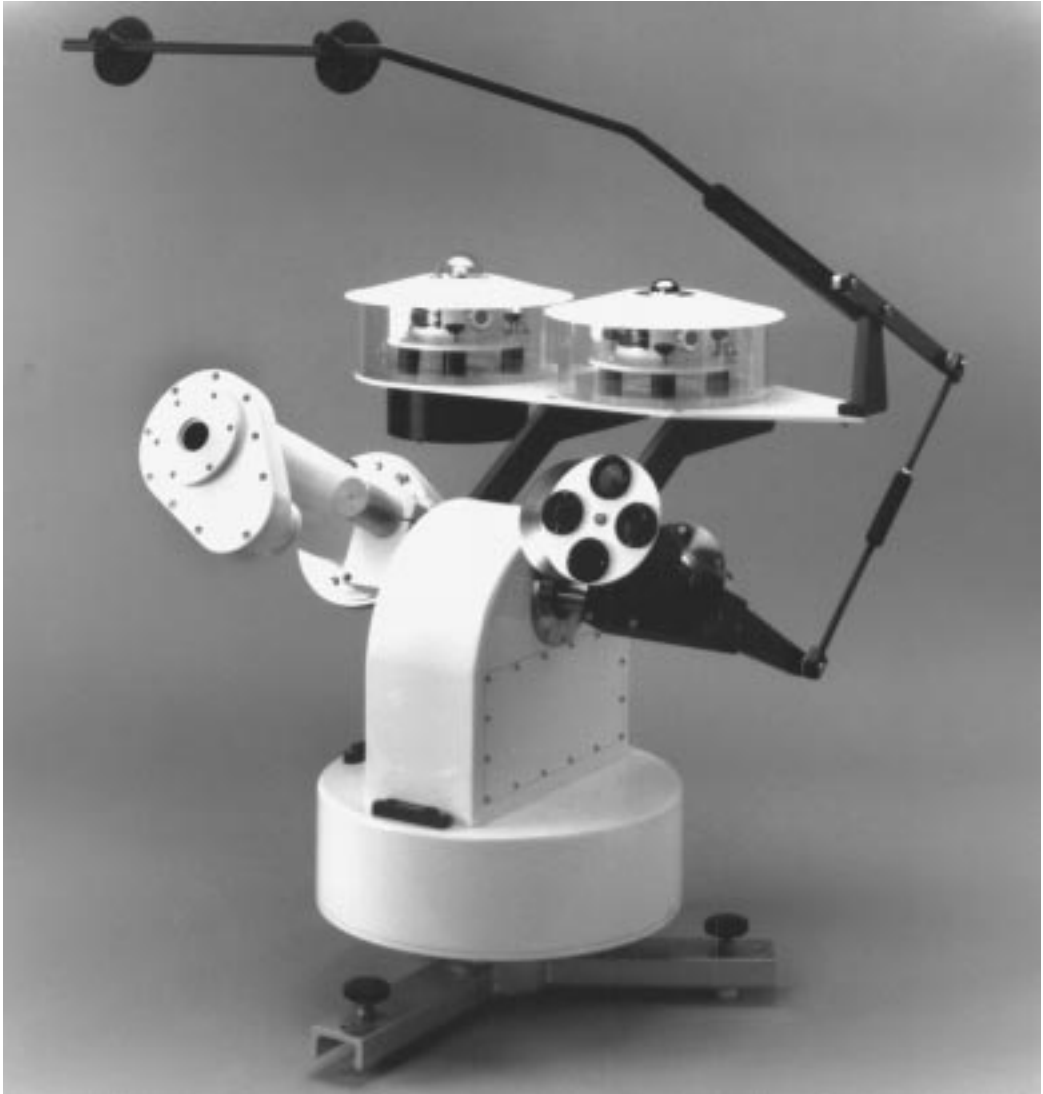
FIGURE 73.4 An automatic solar tracker with normal incidence pyrheliometer and cavity radiometer mounted on it. The tracker is coupled to two shade disks that shield direct sunlight from a first class pyranometer and precision infrared radiometer facing the sky hemisphere. (Courtesy of Eppley Laboratories.)
