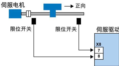
The diagram illustrates a servo motor system. A servo motor is connected to a shaft with a blue T-shaped stop. Two limit switches are mounted on the shaft: one on the left (labeled '限位开关') and one on the right (labeled '限位开关'). The right limit switch is connected to pin X8-7 of the '伺服驱动' (servo drive) unit. The left limit switch is connected to pin X8-8 of the same unit. An arrow labeled '正向' (forward) points to the right, indicating the direction of travel.
