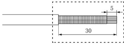
去除电缆的外护套 30 mm
