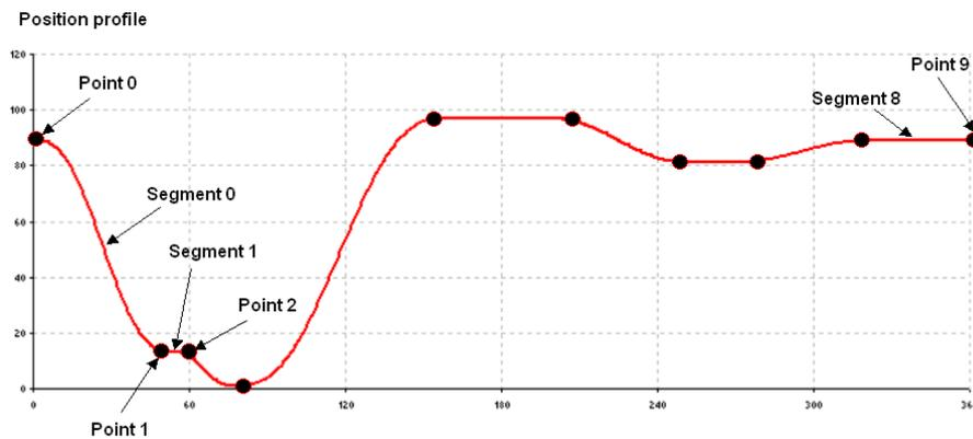
To define the cam segments all points and their dynamics (1<sup>st</sup> and 2<sup>nd</sup> geometric derivation) have to be specified.
