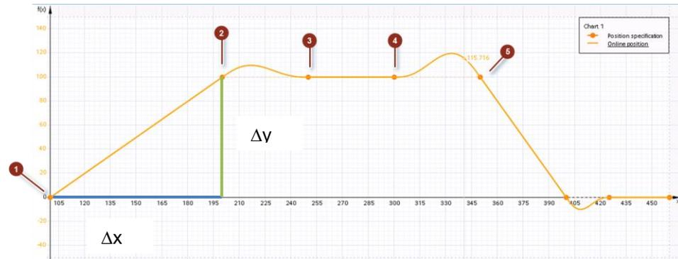
Figure 4-2: Configuration of cam with 8 points created by *LCamHdl\_CreateCamBasic*
