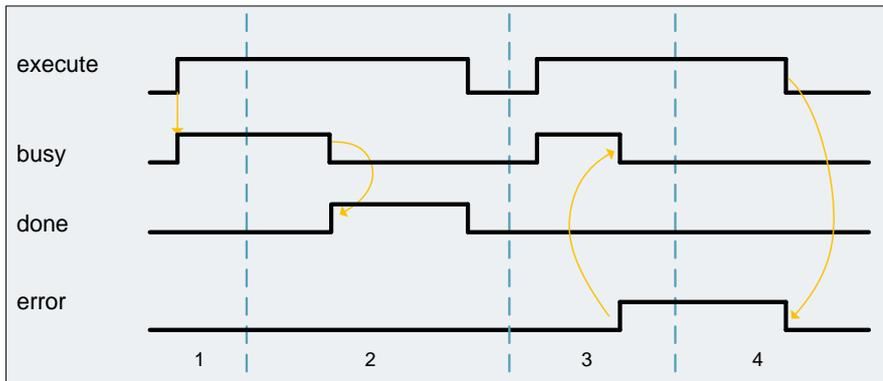
1. The function block is activated by setting the *execute* input. The processing of the FB is indicated with *busy* = TRUE and *done* = FALSE.
