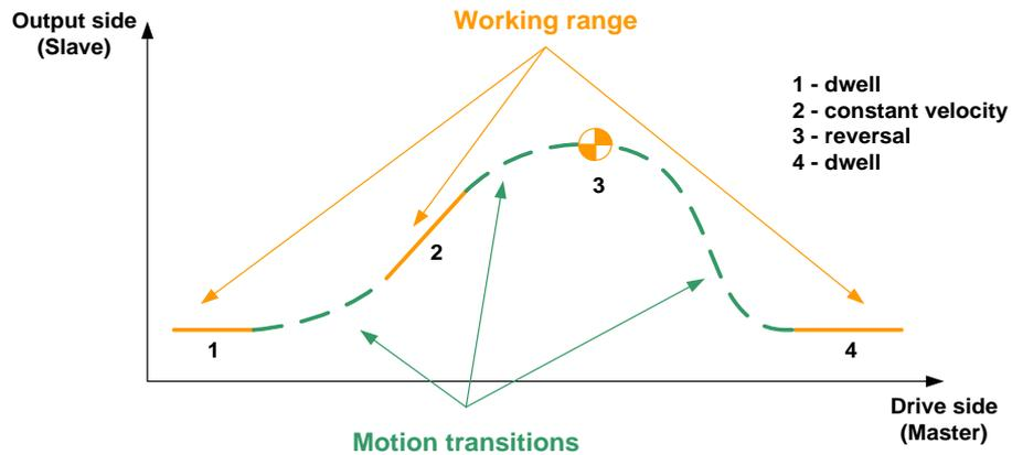
A motion transition between two consecutive working ranges has to fulfill boundary conditions (Figure 4-7), e.g. velocity and acceleration has to be continuous. This guarantees that the drive runs smoothly, e.g. without jerks. The elements are described by mathematic functions between start and end point, e.g. polynomials.
