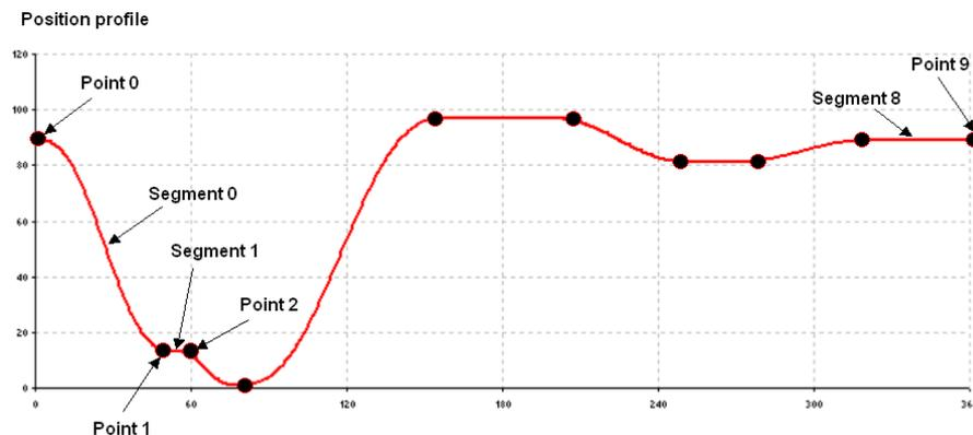
If the working ranges change during the operation of a machine by, for example, a changed length of the product, it is necessary to adapt the motion transitions as well.
