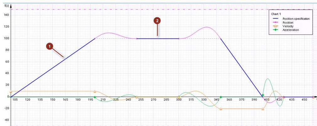
Figure 1-5: Configuration of cam with 4 segments created by CamHdl\_CreateCamAdvanced
