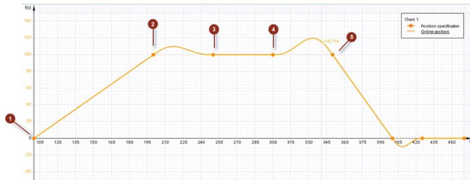
Figure 1-3: Configuration of cam with 8 points created by LCamHdl\_CreateCamBasic
