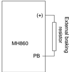
Braking unit installation
