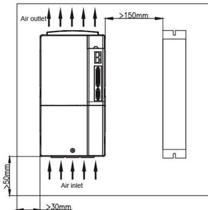
Figure 10-1 MH860-018/025/032/038/043/060/070/092/115 drive and braking resistor layout (mm)
