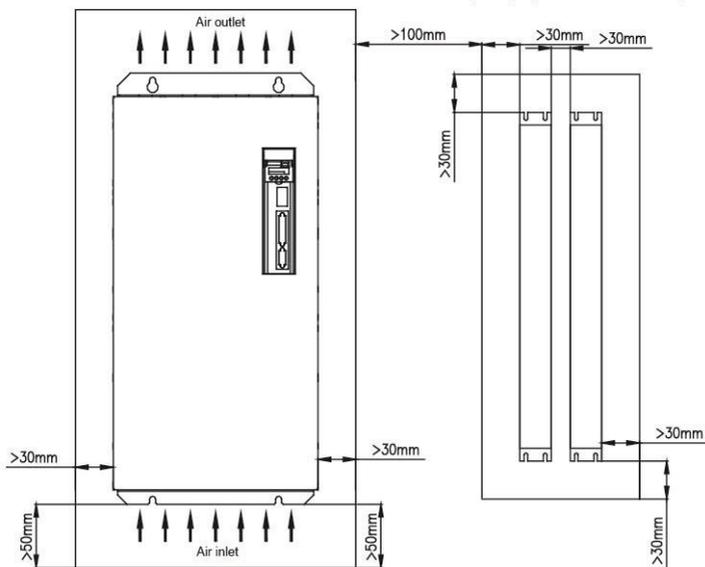
Figure 10-2 MH860-150/170/180/215 drive and braking resistor layout (mm)
