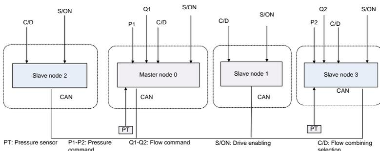
Example: The hydraulic system has four oil pumps, with the addresses set to 0, 1, 2, and 3. There may be two types of action combination:
