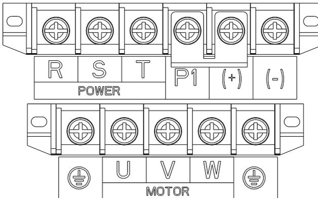
Figure 4-5 Terminal diagram of the 110kW main circuit
