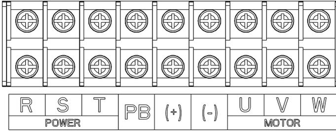
Figure 4-3 Terminal diagram of the 45kW–55kW main circuit
