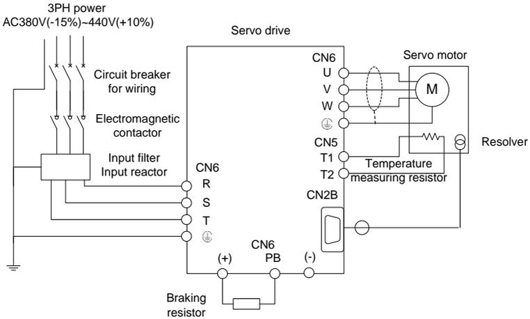
Figure 4-9 Wiring diagram of  $\leq 90\text{kW}$  main circuit
