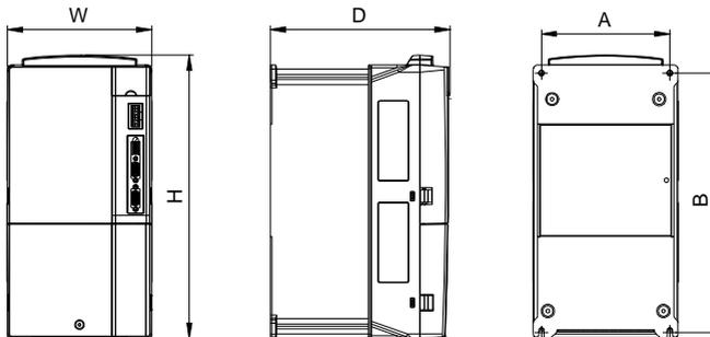
Figure 2-1 Dimensions of MH860-T018SF7-T070SF7
