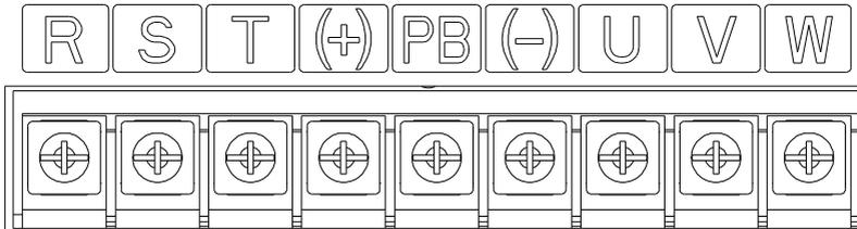
Figure 4-2 Terminal diagram of the 30kW–37kW main circuit
