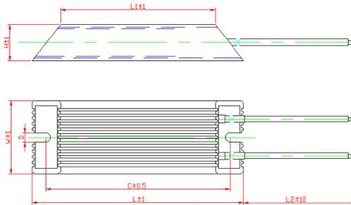
The aluminum-housed braking resistors RXLG-2000W-10RJ (for 092/115 drives, or for two of 150/170/180 drives in parallel connection), and RXLG-2000W-30RJ (for two of 215 drives in parallel connection) are as follows.
