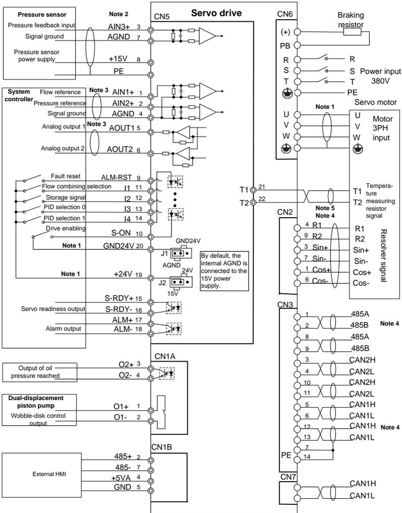
**Note 1:** In this wiring diagram, digital input signal uses the internal 15V power supply of the drive by default. If you want to use an external power supply, connect J2 to the GND24V side and connect J2 to the 24V side to perform the power supply switchover.
