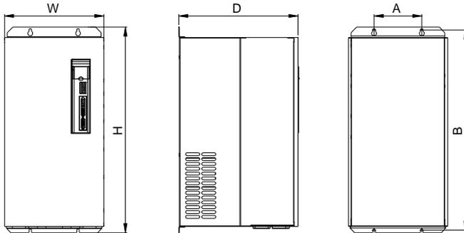
Figure 2-2 Dimensions of MH860-T092SF7-T215SF7
