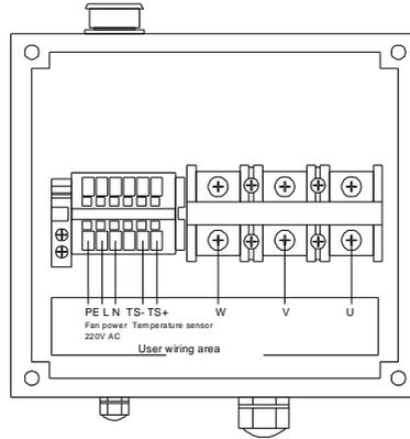
Figure 4-8 Motor wiring terminals
