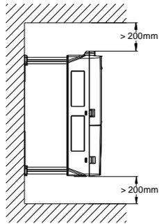
Figure 3-1 Drive installation diagram
