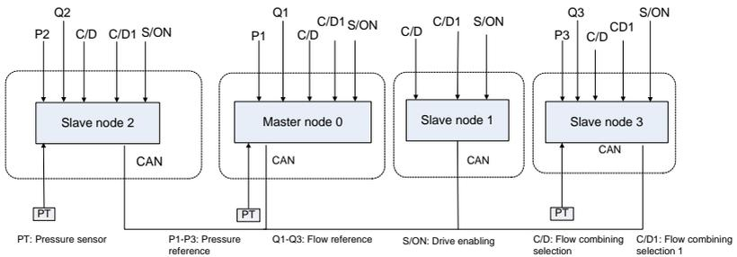
Example: The hydraulic system has four oil pumps, with the addresses set to 0, 1, 4, and 3. There may be two types of action combination:
