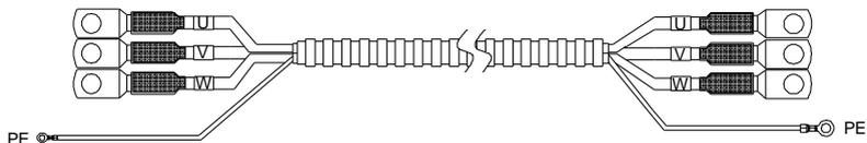
Figure 4-7 Motor power cable
