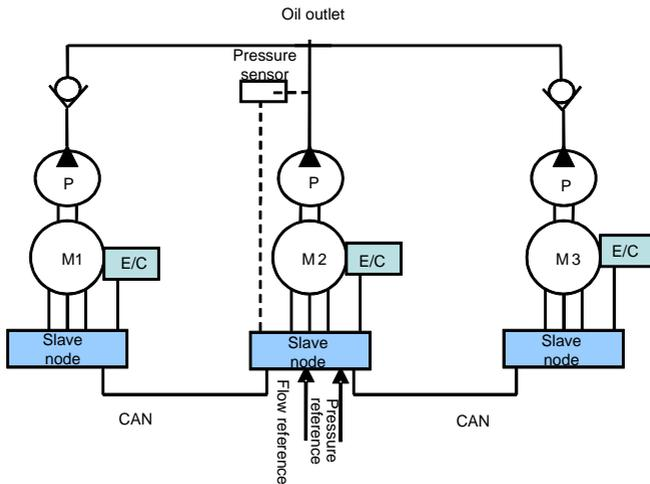
2. Multi-pump wiring diagram:
