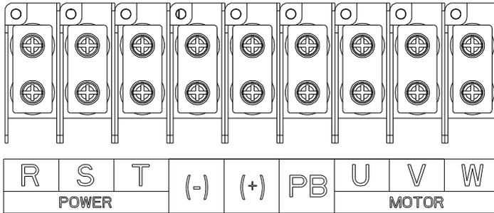
Figure 4-4 Terminal diagram of the 75kW–90kW main circuit
