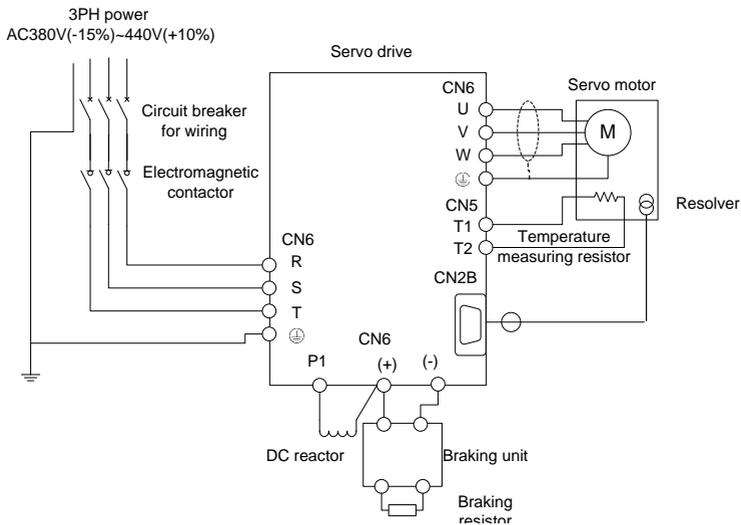
Figure 4-10 Wiring diagram of  $\geq 110\text{kW}$  main circuit
