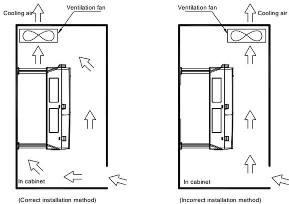
Figure 3-2 Ventilation fan installation position
