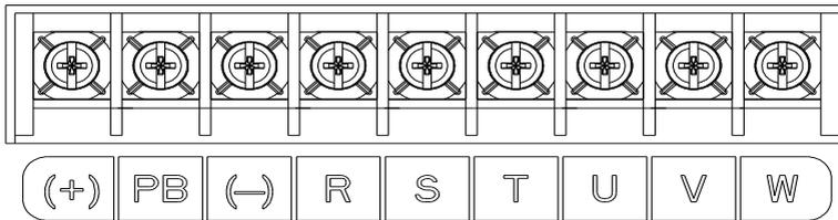
Figure 4-1 Terminal diagram of the 7.5kW–22kW main circuit
