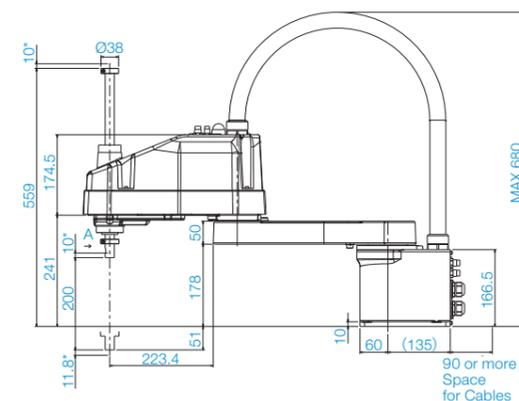
\*indicates the stroke margin by mechanical stop.
