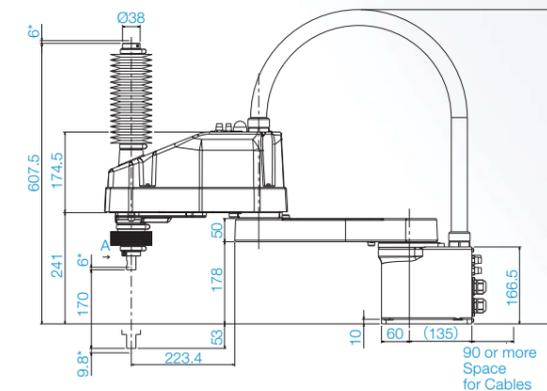
\*indicates the stroke margin by mechanical stop.
