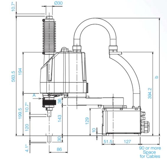
\*indicates the stroke margin by mechanical stop.
