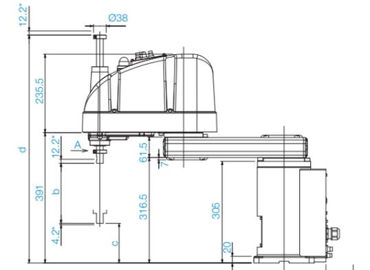
\* indicates the stroke margin by mechanical stop.
