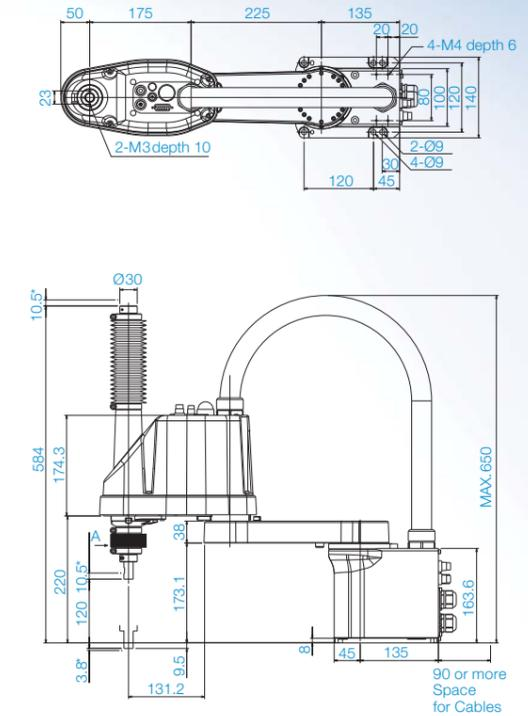
\*indicates the stroke margin by mechanical stop.
