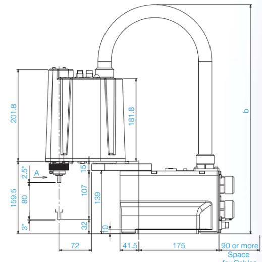
\*indicates the stroke margin by mechanical stop.
