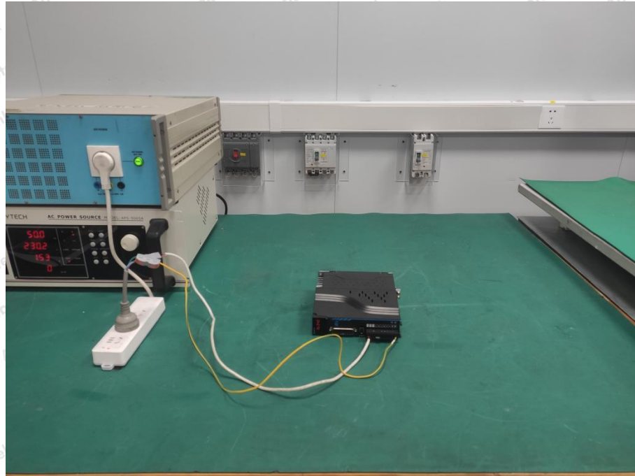
Photo of Harmonic Current And Flicker Test
