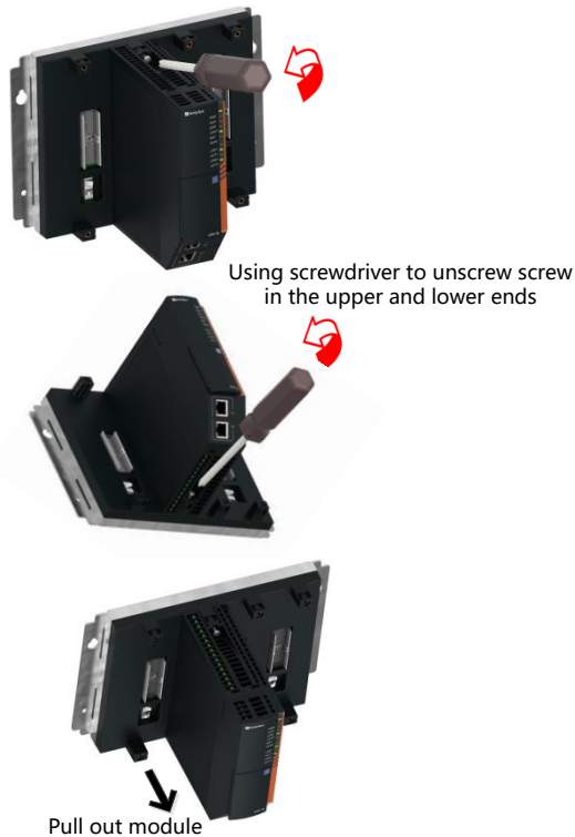
Figure 12 Dismantle Module
