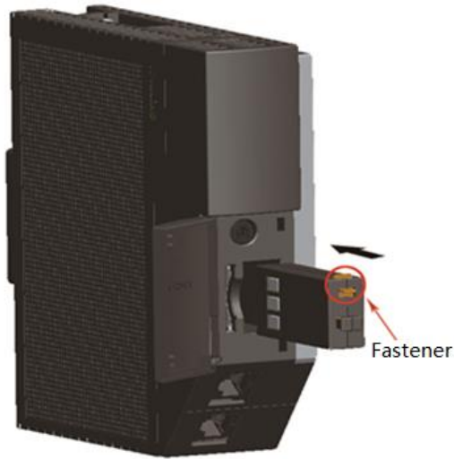
Figure 19 Installation Schematic Diagram of Power Supply Box
