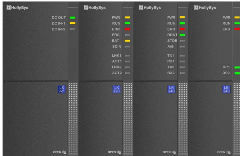
Figure 395 Abnormal Indicator Diagram
