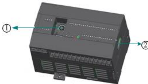
Figure 79 Communication Interface Identification
