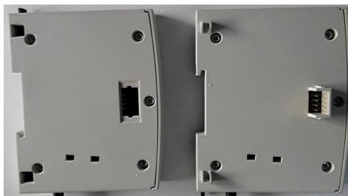
Connection box on the lower side of expansion cable    Connection box on the upper side of expansion cable
