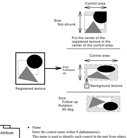
This name is used to identify each control in the part from others. If the part operation program is already created, the control name is referenced by the program. Thus, be careful not to change any control name unnecessarily. Otherwise, the change will affect the program badly. Action
