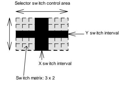
Sw itch matrix setup Number of sw itch ream step: 2 x 2 X sw itch interval: 2 Y sw itch interval: 1 Attribute
