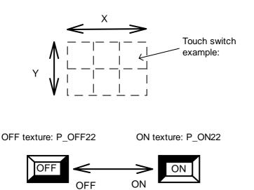
When both ON and OFF texture are specified, the switch texture is displayed according to the switch ON/OFF status.
