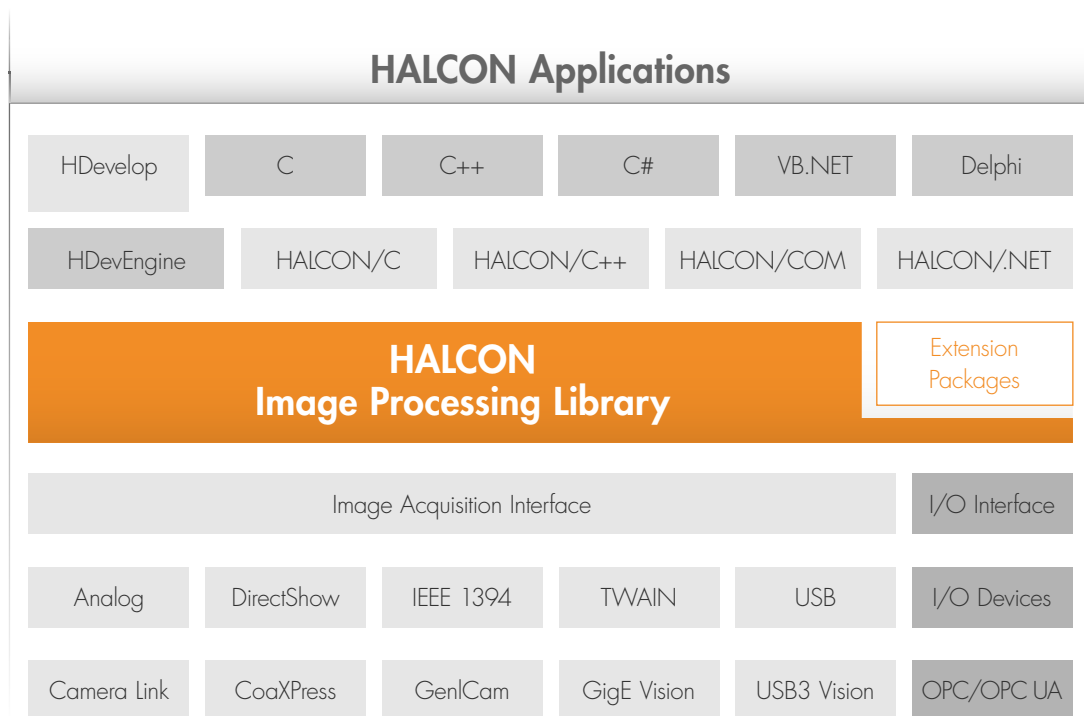
Figure 2.2: Basic architecture of HALCON.
