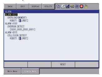
The following operations are available in the alarm status: window change, mode change, alarm reset, and emergency stop. To display the ALARM window again when the window is changed during alarm occurrence, select {SYSTEM INFO} and then {ALARM HISTORY}.
