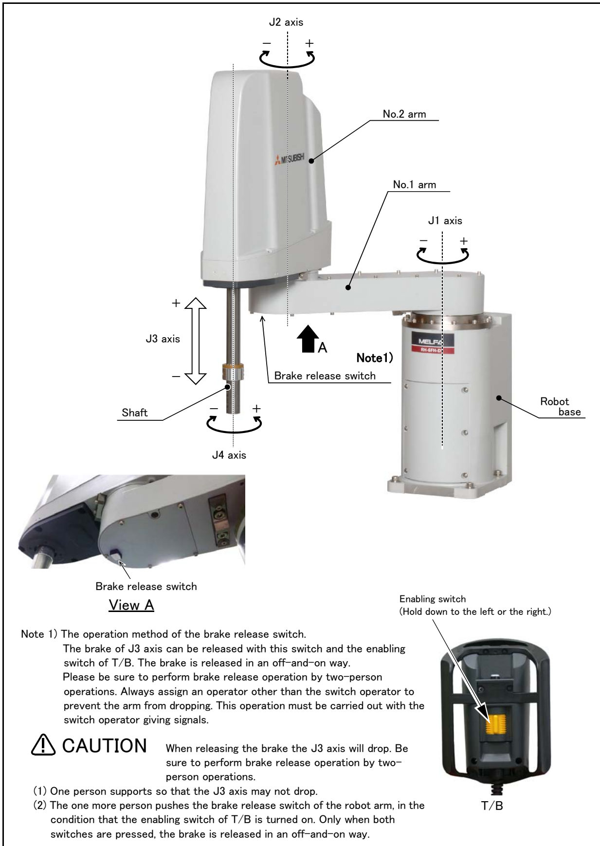
Fig.2-11 : Names of each part of the robot
