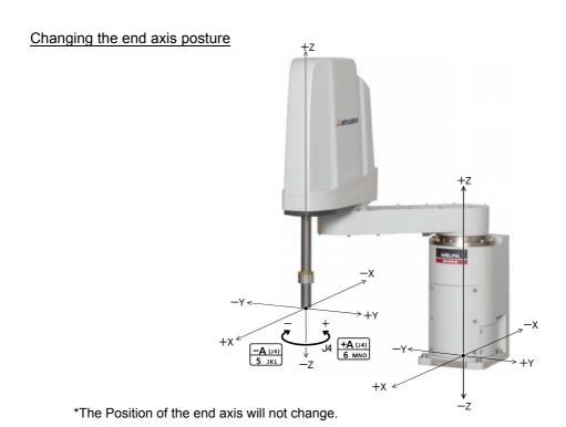
• When the [+C (J6)] keys are pressed, the J4-axis will rotate in the plus direction. When the [-C (J6)] keys are pressed, Rotate in the minus direction.
