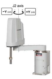
• When the [+Y (J2)] keys are pressed, the J2 axis will rotate in the plus direction. When the [-Y (J2)] keys are pressed, Rotate in the minus direction.
