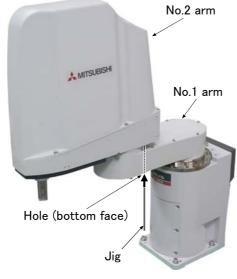
2) Slowly rotate the J2 axis, and align the pinholes of the No. 1 and No. 2 arms, feed through the origin jig into the pinholes and fasten.
