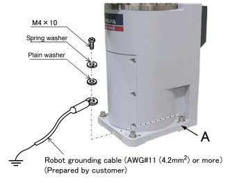
Fig.2-6: Connecting the grounding cable
