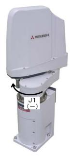
2) With both hands, slowly move the J1 axis in -(minus) direction, and contact the axis against the mechanical stopper.
