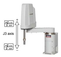
• When the [+Z (J3)] keys are pressed, the J3 axis will rotate in the plus direction. When the [-Z (J3)] keys are pressed, Rotate in the minus direction.
