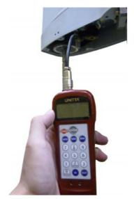
Image of Measurement by the sound wave type belt tension gauge
