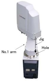
2) Move the J1 axis slowly toward the front using both hands. Align the pinhole of the No.1 arm and the pinhole at the base section, feed through the origin jig into the pinholes and fasten.
