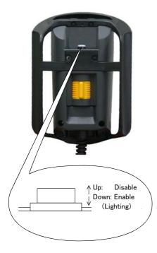
2) Set the T/B [ENABLE] switch to "ENABLE". The menu selection screen will appear.
