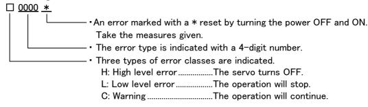
The axis No. may be indicated at the last digit of the error No. Example) H0931 No. 1 axis motor overcurrent.
