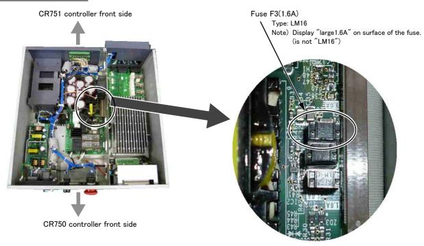
Fig.2-1: Fuse exchange place
